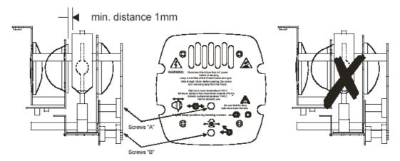
The **POWER WASH 250™** lamp holder is aligned at the factory. However, due to slight imperfections in all lamps, fine adjustments may improve light performance. Please follow this procedure:
