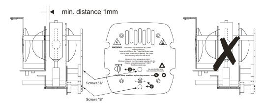
The **POWER SPOT 250™** lamp holder is aligned at the factory. However, due to slight imperfections in all lamps, fine adjustments may improve light performance. Please follow the procedures below to properly fine-tune the lamp orientation:
