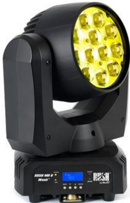
The RUSH MH 6 Wash is an exciting adaption of the hugely popular RUSH PAR 2 RGBW Zoom, using the same LED engine and zoom system, but additionally featuring moving head capability. The RUSH MH 6 Wash offers a fully pre-mixed color system from 12 x 10 W RGBW LEDs with a spectacular 10°–60° zoom. It also offers full electronic dimming, strobe effects and temperature-controlled fan cooling for quiet operation.
