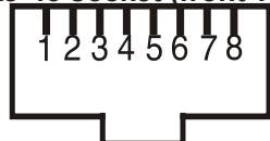
RJ-45 socket (front view):
