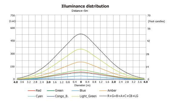
Fixture settings: DMX Mode: 3 Colour calibration mode: On Colour mixing mode: RGB Output mode: Intensity Theatre mode: Off
