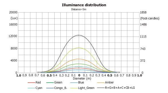
Fixture settings: DMX Mode: 3 Colour calibration mode: On Colour mixing mode: RGB Output mode: Intensity Theatre mode: Off
