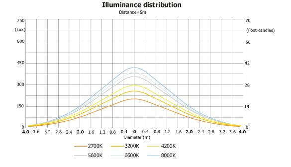
Fixture settings: DMX Mode: 3 (R+G+B+A+C+CB+LG=full) Colour calibration mode: On Colour mixing mode: RGB Output mode: CRI Output Uniformity: On Output Consistency: 50°C CRI Selection: 90+ Theatre mode: Off
