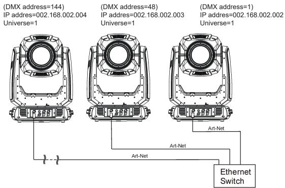
An advised PC setting: IP address: 002.xxx.xxx / 010.xxx.xxx (Different from fixture IP addresses) NET mask: 255.0.0.0
