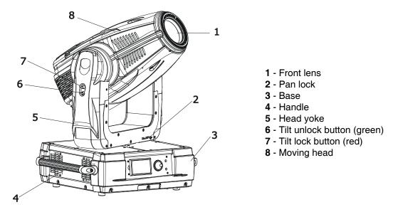
The head should be locked for transportation- the tilt lock button (7) is pushed and the pan lock/unlock lever (2) is in locked position. To unlock the head, press the tilt unlock button (6) and move the pan lock/unlock latch (2) into unlocked position.
