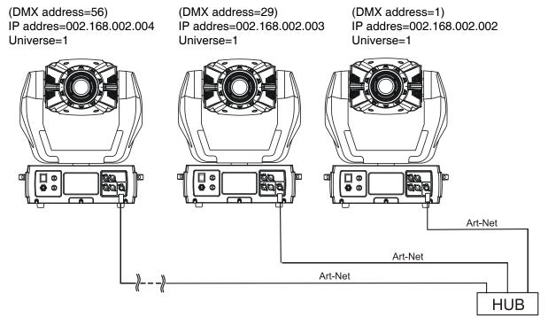
An advised PC setting: IP address: 002.xxx.xxx / 010.xxx.xxx (Different from fixture IP addresses) NET mask: 255.0.00
