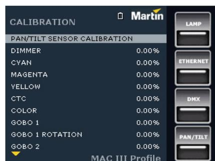
**Warning!** As soon as you exit pan/tilt sensor calibration, the head will move to its original position.
