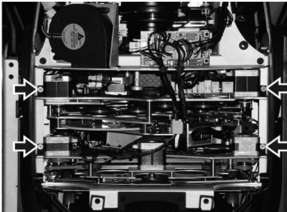
Figure 27: Module retaining screws
