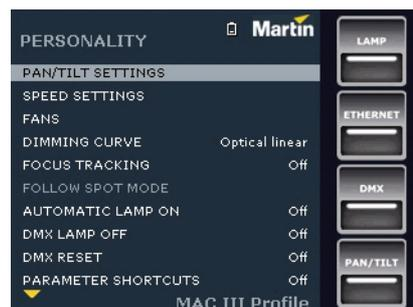
Pan range for pan limit purposes runs from 0° to 360° clockwise as seen looking at the fixture from the bottom of the base towards the yoke, as if the fixture was hanging downwards underneath you. Tilt range is +134° and -134° either side of 0°, which is the head straight up position with the front glass pointed directly away from the base.
