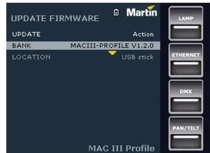
Zoom-focus linking is reset to default (medium distance) when new software is uploaded. Other fixture information and settings are unaffected.
