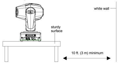
Figure 7-23. Orient the fixture for lamp optimization.
