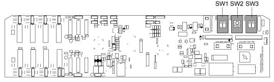
Figure 1-5. Circuit board containing the three switch blocks.
