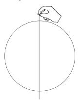
Extend the tape measure or ruler across the horizontal center of the beam and lightly mark the center of the beam on the wall along the ruler
