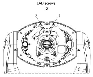
Figure 6-7. LAD™ mounting/alignment screws.
