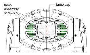
Figure 7-5. Lamp cap and lamp assembly screws.
