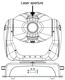
Figure 6-2. Laser aperture.
