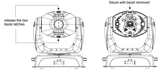
Figure 1-1. Removing the bezel.
