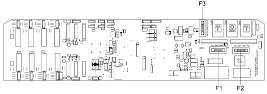
Figure 7-4. Fuses on the circuit board.
