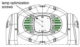
Figure 7-24. Lamp optimization screws.
