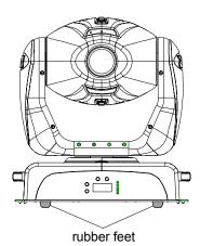
Figure 1-13. Rubber feet on the fixture.
