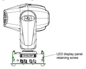
Figure 7-2. Loosen the two display panel retaining screws.
