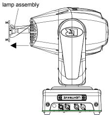
Figure 7-6. Remove the lamp assembly.
