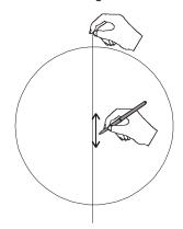
4 Measure 3.3 in (8.4 cm) for Studio Spot 250 fixtures, or 3.5 in. (8.9 cm) for Studio Color 250 fixtures above the center point of the marks you made on the wall to mark where the laser should shine.
