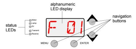
Figure 1-7. Front panel display.
