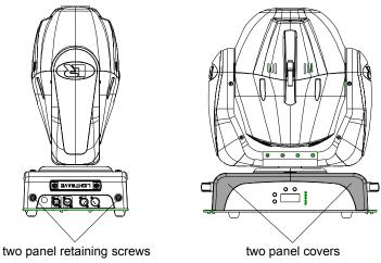
Figure 7-1. Remove the two panel covers.
