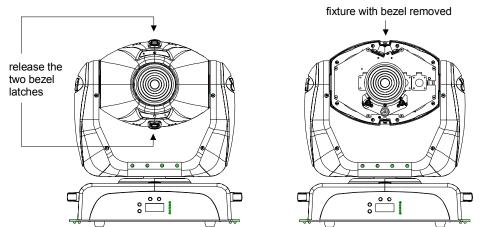
Figure 7-17. Remove the fixture's bezel.
