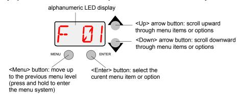
Figure 4-1. Use the <Menu>, <Enter>, <Up>, and <Down> keys to navigate through the menu system.
