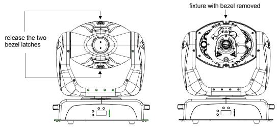
Figure 6-5. Remove the bezel.
