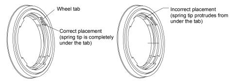
Figure 7-16. Replacing the spring on a rotating litho or effect.
