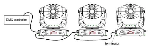
Figure 1-11. Linking the fixtures.
