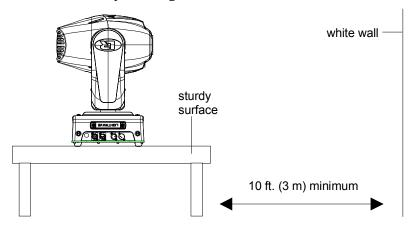
Figure 6-4. Orient the fixture for laser alignment.
