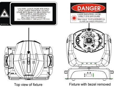
Figure 6-1. LAD<sup>™</sup> labels on the fixture.
