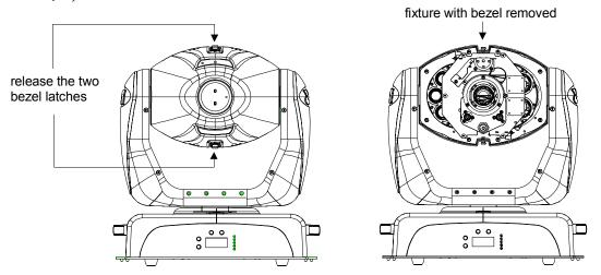
Figure 7-8. Remove the fixture's bezel.
