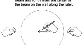
2 Lightly mark the center of the beam on the wall along the ruler.
