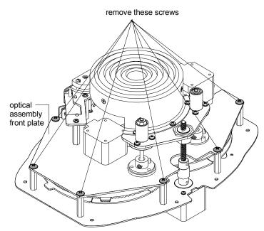
Figure 7-19. Location of the eight screws on the optical assembly front plate.
