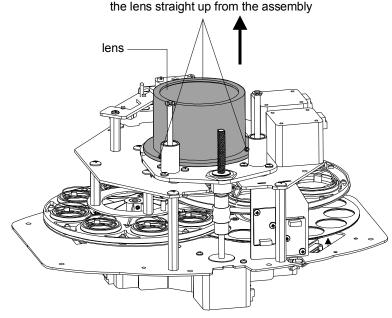
remove the three lens screws and pull
