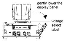
Figure 1-4. Lower the display panel.
