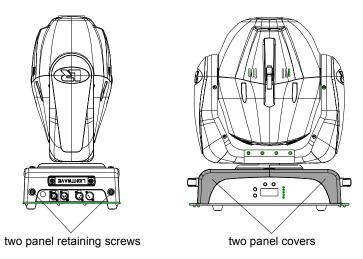
Figure 1-2. Remove the two panel covers.
