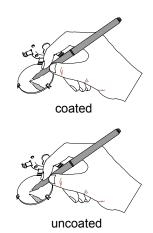
Figure 7-11. Determining the coated side of dichroic glass.
