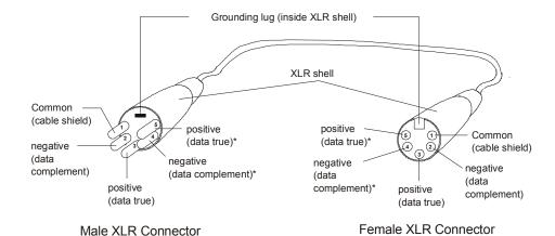
\*This data line is not used by the fixture, but allows data to pass through the fixture.
