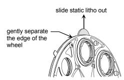
Figure 7-14. Removing a static litho.
