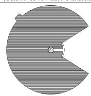
Figure 3-4. Studio Color® 250 beam shaping (lenticular) wheel.
