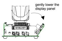
Figure 7-3. Lower the display panel.
