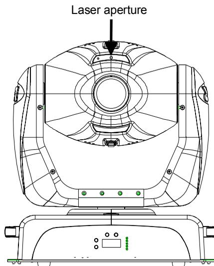
Figure 6-2. Laser aperture.
