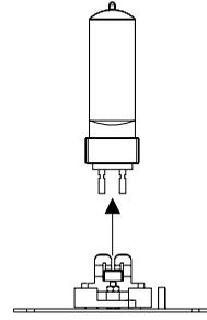
*Figure 7-7. Remove the lamp from the lamp socket.*
