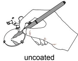
Figure 7-11. Determining the coated side of dichroic glass.
