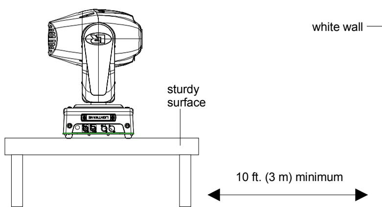
Figure 7-23. Orient the fixture for lamp optimization.
