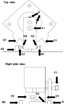
properly. Re-adjustment of the Pan or Tilt dampers is necessary if the end-stop adjustments have caused either of the motors to slide along its axis at any time.
