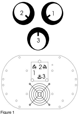
If you are not satisfied with the light-output you can try to adjust the lamp-holder further by turning all of the screws a 1/4 turn clockwise, making
