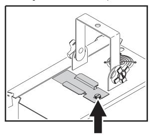
3 Lift the gobo holder out of the fixture.
