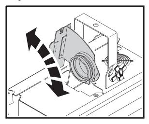
4 The gobo/texture glass is held in place by a steel spring. Remove the spring to remove the gobo/texture glass that is presently installed.
