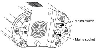
2 Turn the power on using the mains switch.
