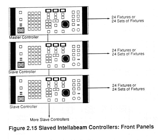
To put a controller in Slave Mode, set Personality DIP switch number one on the rear panel of the controller to the "ON" or up position.
