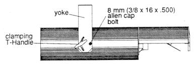
Figure 2.1 Intellabeam Fixture: Side View
