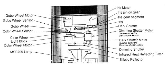
Figure 7.1 Intellabeam Fixture: Top Access Door Removed
