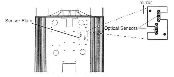
Figure 7.7 Intellabeam Fixture: Bottom Door Removed
