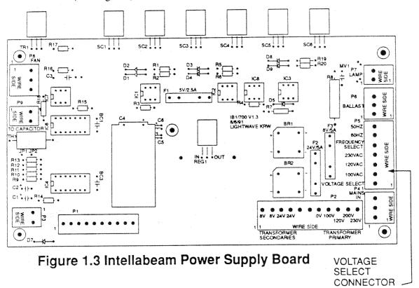
• You can remove the connector, or you can change the jumpers while the connector is still in the fixture.
