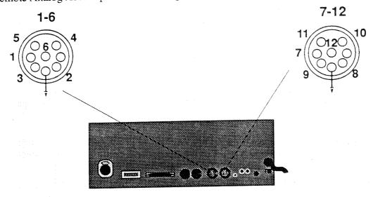
Figure 5.1 Pinout of Remote Access Ports
