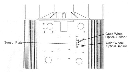
• Locate the two screws which hold the sensor plate in place. (See Fig.7.2.)
