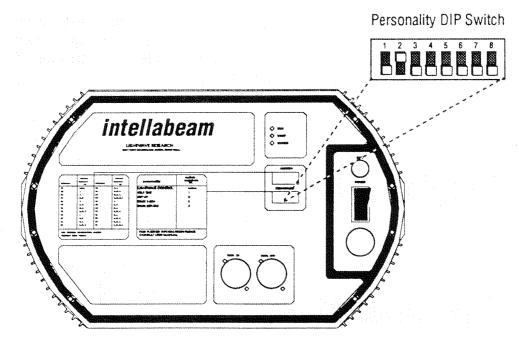
Figure 2.6 Intellabeam Fixture: Rear Panel
