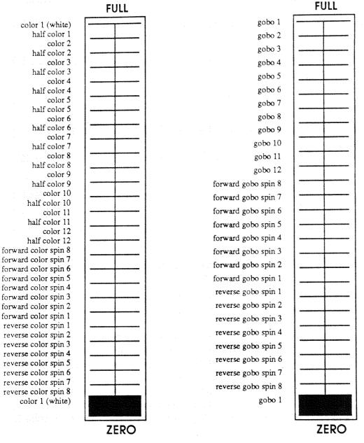
Figure 2.9 DMX Faders with High Resolution Capabilities
