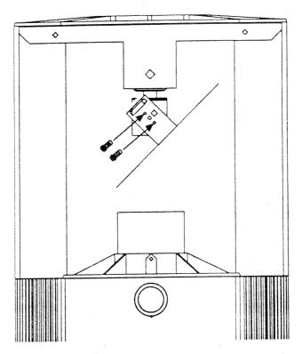
Figure 7.8 Intellabeam Fixture: Mirror Installation
