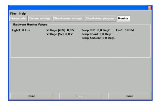
Light1 displays the light level currently measured by light sensor 1 on the back of the fixture.
