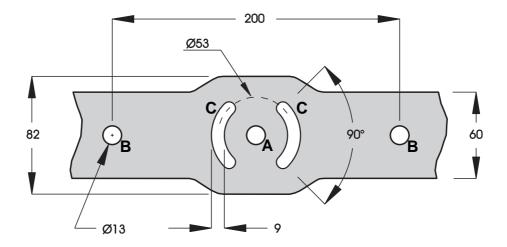
Figure 1: Mounting yoke attachment points
