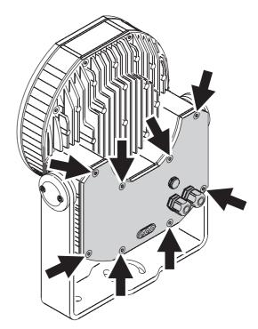
Figure 4: Rear cover retaining screws
