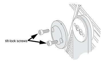
Figure 2: Tilt adjustment
