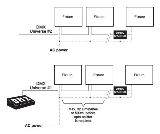
Figure 3: Schematic cable layout diagram
