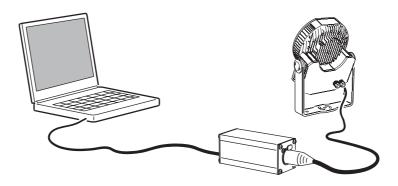
Figure 10: Connecting to a PC with MUM
