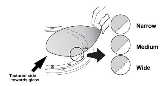
Figure 18: Installing a diffuser filter
