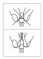
**DISCHARGE LAMP WARNING:** This fixture is fitted with a discharge lamp, which is highly susceptible to damage if improperly handled. Never touch the lamp with your bare hands, as the oil from your hands will shorten lamp life. Also, never move the fixture until the lamp has had ample time to cool. Remember, lamps are not covered under warranty conditions.
